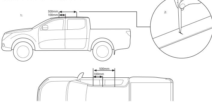
Step 2 Centre the correct brackets over the marks made in the last step. Mark the width of the brackets onto the ditch fill.
