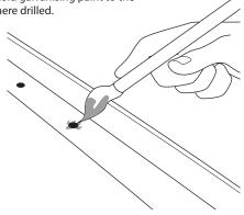
Apply cold galvanising paint to the underside of the roof where drilled.
