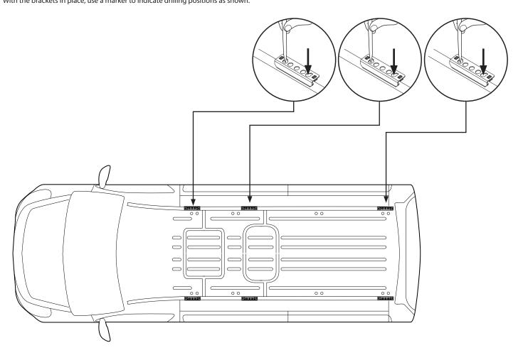
Pilot drill with a 3mm bit, then using a 6.5mm drill bit and a depth gauge set to 5mm, carefully drill through your roof references. **Note:** It is advised to drill the rear left and front left bracket with assistance. Loom wiring is present under these drilling locations. Apply tape in the approximate drilling location to capture swarf. An
