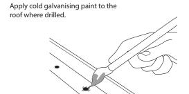
Apply cold galvanising paint to the underside of the roof where drilled.
