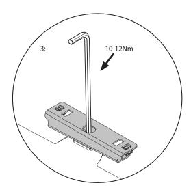
ATTENTION: Bracket orientation is critical. Note the number of M8 spacer washers used:
