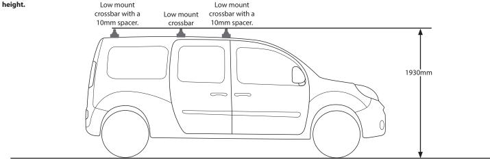
Note: No spacers are required for a 2 bar setup:
