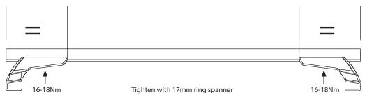
Step 4 Note: If rubber is too long, cut to length. Insert end caps and rubber strips. Observe the orientation of the end caps. Leave a 10mm overhang, this will compress under the end cap.
