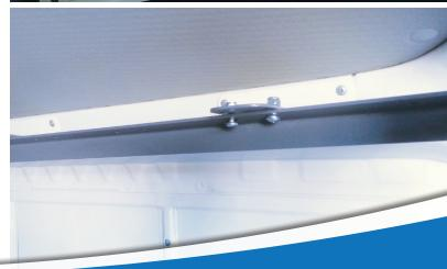
**Step 15:** Using a P3 Phillips Head bit, attach the bottom shelf to the VAS Shelving System frame using 8 X Dog Head screws.
