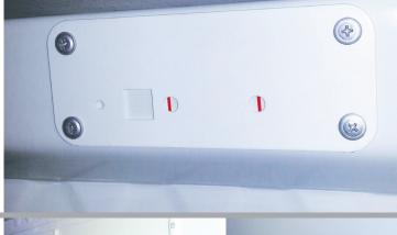
**Step 8:** Drill holes using a 7.5mm drill bit (if you do not have a drill stop you can use tape around the drill bit, as show in the image to the right). This is to prevent you from drilling through to the outside of your vehicle.
