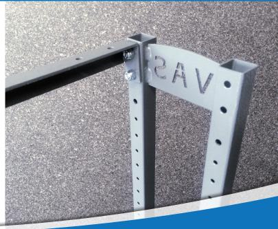
**Step 2:** Attach the pivot 'U' bracket to the pivot arm using 2 X ¼" x 5/8" bolts and ¼" Nyloc nuts, to use as marking template.
