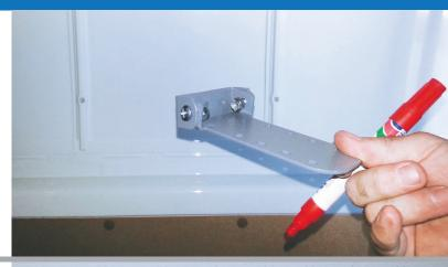
**Step 3:** Line up the holes in pivot plate with the holes in the VAS Shelving System crossbar. With a marking pen, mark where the holes in the pivot 'U' bracket locate on the cant rail in your vehicle. Try to stay clear of the joins in panels.
