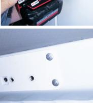
**Step 9:** Using a step drill (if you don't have a step drill you can use a 16mm hole saw), drill out the larger square hole to fit the insert plate through.
