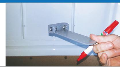
**Step 3:** Line up the holes in pivot plate with the holes in the VAS Shelving System crossbar. With a marking pen, mark where the holes in the pivot 'U' bracket locate on the cant rail in your vehicle. Try to stay clear of the joins in panels.
