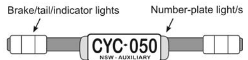
Example of duplicate vehicle lights, in this case fitted to a detachable bar
